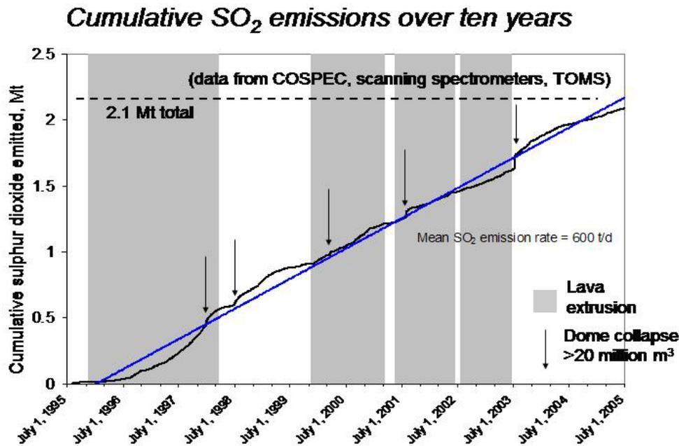
Fig. 2 Cumulative sulphur dioxide emissions to the atmosphere 1995-2005, blue line is best linear fit ( from Edmonds, 2005)
