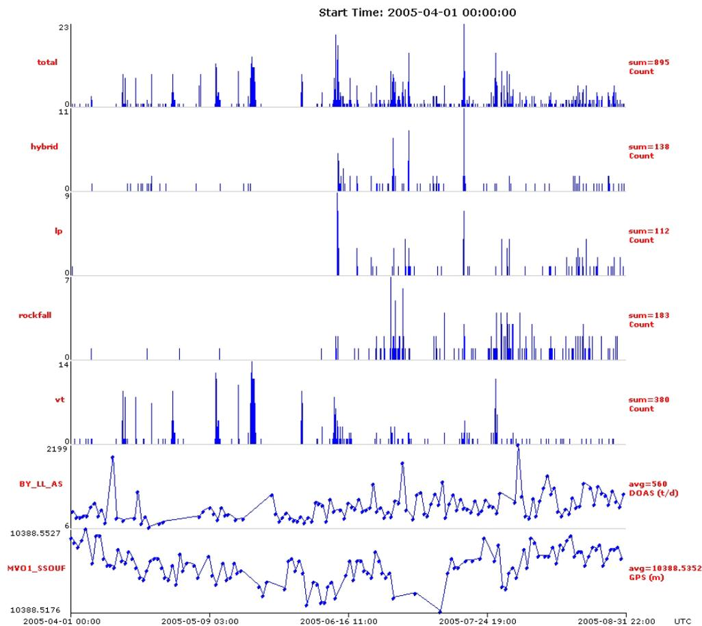
Fig.1 MVO plots of seismicity, gas and deformation data for April to September 2005. The plots are from the top: numbers of all seismic events, hybrid events, long-period events, rockfalls, volcano-tectonic events, daily sulphur dioxide emission rates and GPS line length changes between MVO1 and SOUF.
