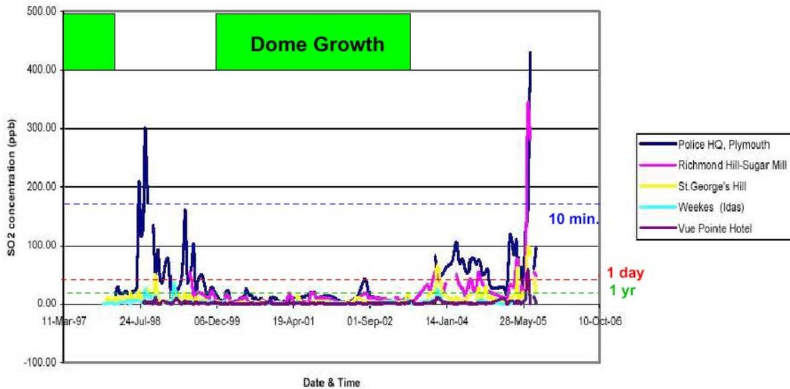
Fig. 4. Cumulative ground level sulphur dioxide concentrations measured by diffusion tubes in and around the former TDEZ from 1997 to 2005.
